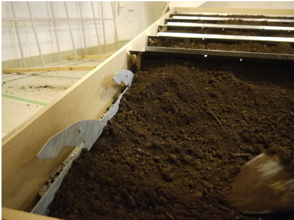
Figure B.1. Assembly of the test set-up: Framework with soil, inside: support profiles with the first plates.
