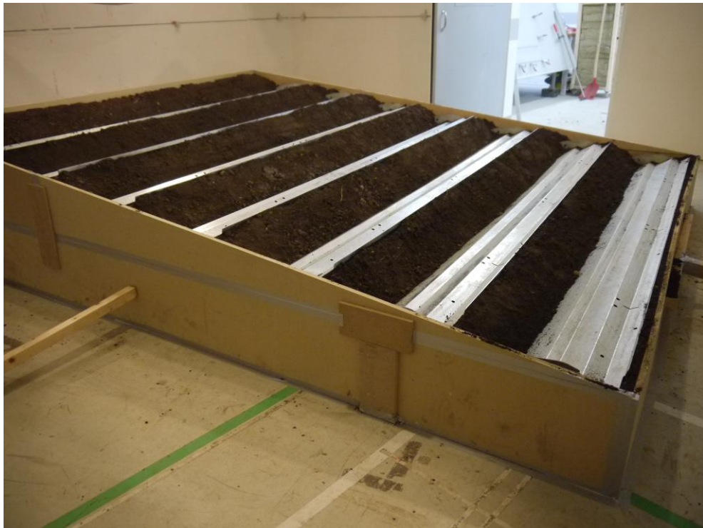
Figure B.3. Test set-up in the reverberation room.
